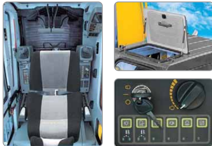
1 Wide, Comfortable Operating Space 2 Steel Cover Sunroof 3 Dial Type Engine Speed Switch and Key Switch
